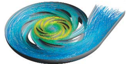
Streamlines shown in cross section through pump impeller, diffuser, and housing of HPB
